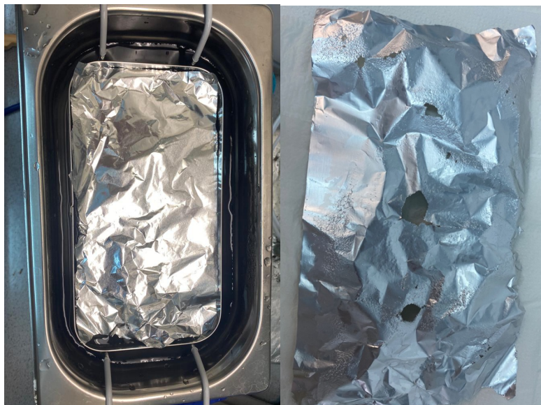
Figure 14: Aluminum foil test on the surface with the stainless-steel basket.
