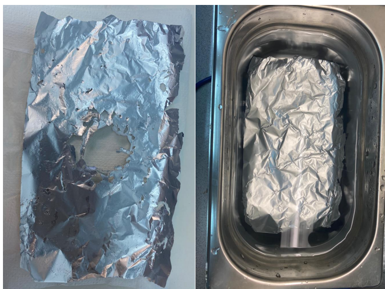
Figure 13: Aluminum foil test at the bottom of the bath without the stainless-steel basket.
